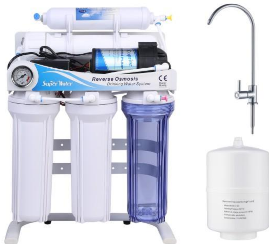
Model KK-RO-07 (Steel Stand with Pressure Gauge) Capacity: 50/75/100GPD Diaphragm Booster Pump with Adaptor 110/220V,50/60HZ RO Membrane: VONTRON or COPRITE Membrane Pressure Tank: 3.2G or 4G plastic Tank
