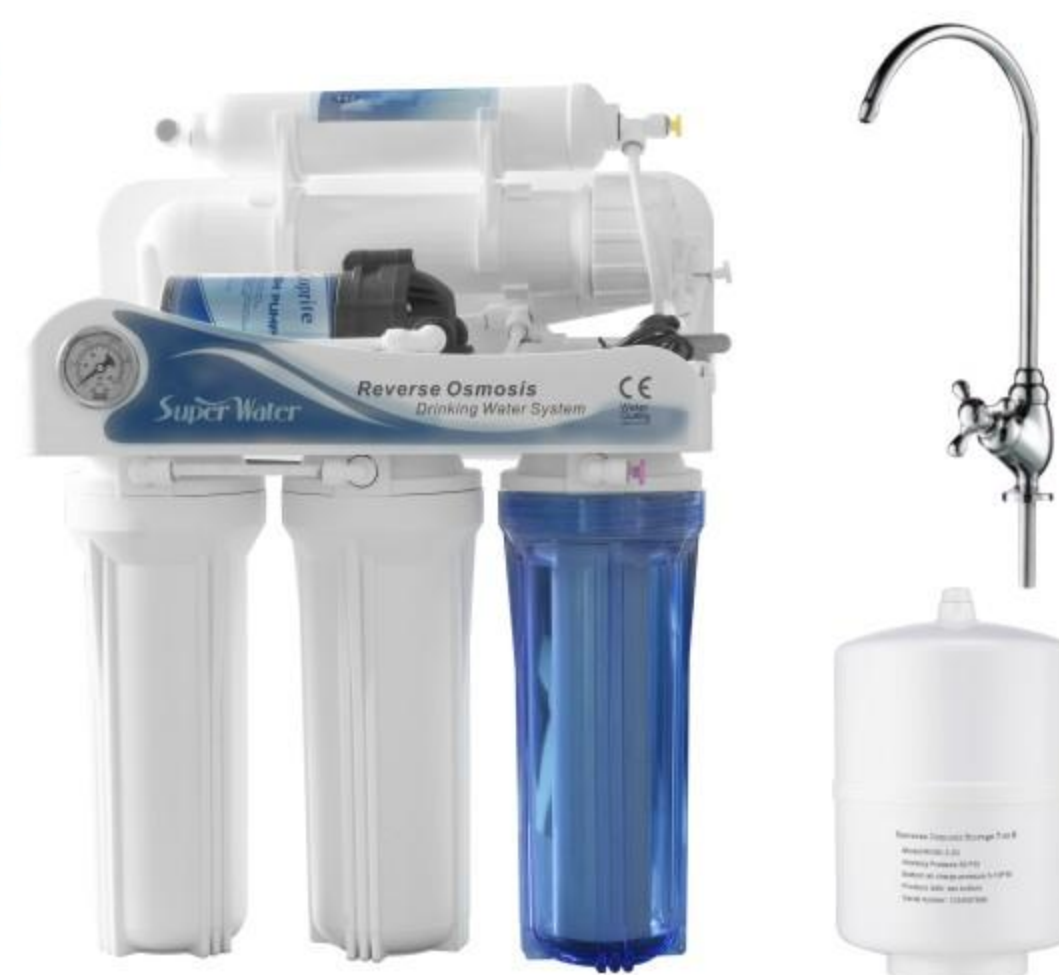
Model KK-RO12 (5-7 Stages with Pressure Gauge) Capacity: 50/75/100GPD Diaphragm Booster Pump with Adaptor 110/220V,50/60HZ RO Membrane: VONTRON or COPRITE Membrane Pressure Tank: 3.2G or 4G plastic Tank
