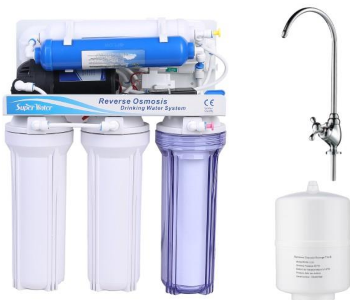
Model KK-RO50G-A (5 Stages) Capacity: 50/75/100GPD Diaphragm Booster Pump with Adaptor 110/220V,50/60HZ RO Membrane: VONTRON or COPRITE Membrane Pressure Tank: 3.2G or 4G plastic Tank
