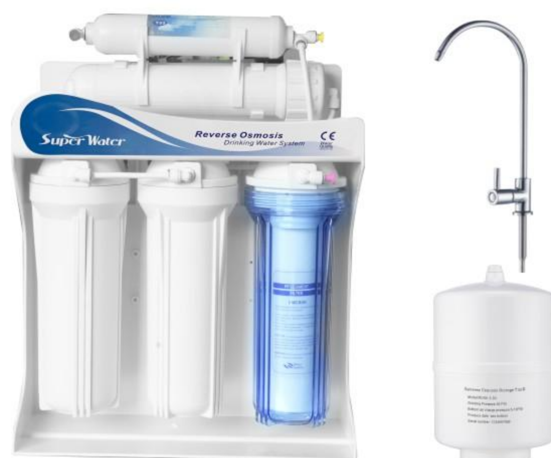
Model KK-RO13 (Plastic Stand) Capacity: 50/75/100GPD Diaphragm Booster Pump with Adaptor 110/220V,50/60HZ RO Membrane: VONTRON or COPRITE Membrane Pressure Tank: 3.2G or 4G plastic Tank
