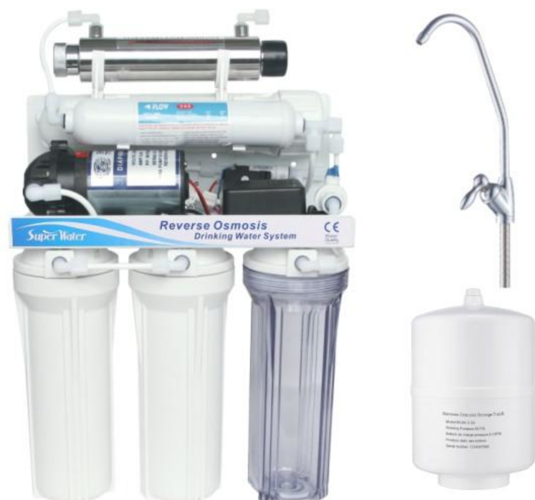
Model KK-RO50G-C (6 Stages with UV) Capacity: 50/75/100GPD Diaphragm Booster Pump with Adaptor 110/220V,50/60HZ RO Membrane: VONTRON or COPRITE Membrane Pressure Tank: 3.2G or 4G plastic Tank
