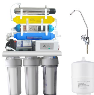
Model KK-RO50G-X (7 stage with UV & computer) Capacity: 50/75/100GPD Diaphragm Booster Pump with Adaptor 110/220V,50/60HZ RO Membrane: VONTRON or COPRITE Membrane Pressure Tank: 3.0G or 4G plastic Tank Unit packing Dimension: 41*35*58cm
